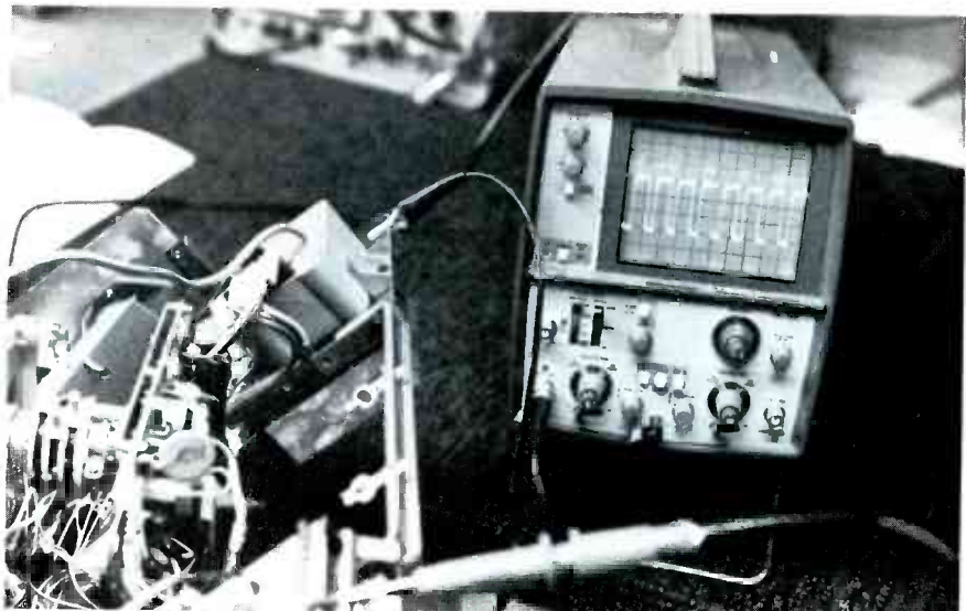
Fig. 8 The scope waveform is correct for the IC201 input signal at the junction of R210 and R211. The amplitude should be between 7 and 11 volts PP (somewhat less at pin 1 of IC201), when a remote button is held down.
