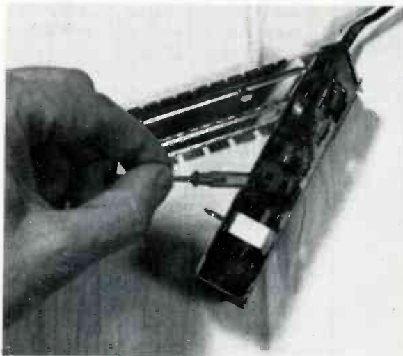
Fig. 13 Some early-production remote amplifiers have one tuned coil (L1). Sometimes the coil picks up an excessive amplitude of pulses from the horizontal-sweep circuit. In such cases, the newer amplifiers without the coil are preferred.
