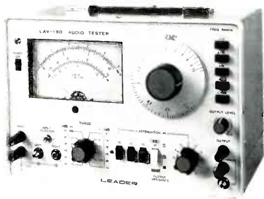
Fig. 1 Leader Model LAV-190 Audio Tester combines the functions of an AC amplified meter (50 microvolts to 500 volts RMS) and an audio generator of sine waves from 10 Hz to 1 MHz, having precision attenuators.
