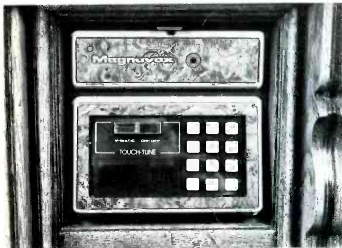
Fig. 2 The "Touch-Tune" panel has pushbuttons for "V-Matic" (a one-button preset-color circuit), a non-locking on/off switch that operates from a digital circuit, and 12 buttons for station selection and control of the sound volume. Space is provided for a remote-control microphone. Remote control can be added at any time.
