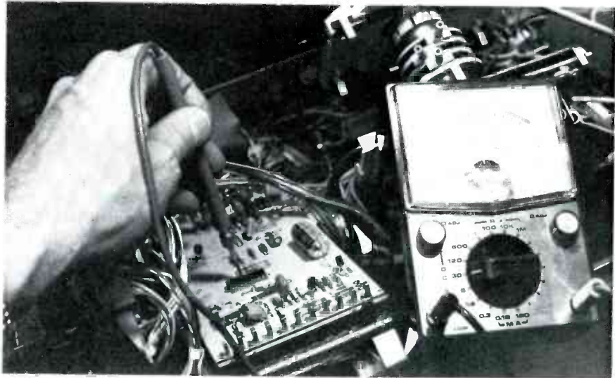
Fig. 7 When high, the outputs of IC201 should measure between +11 and +12 volts. This is an important test of the operation.
