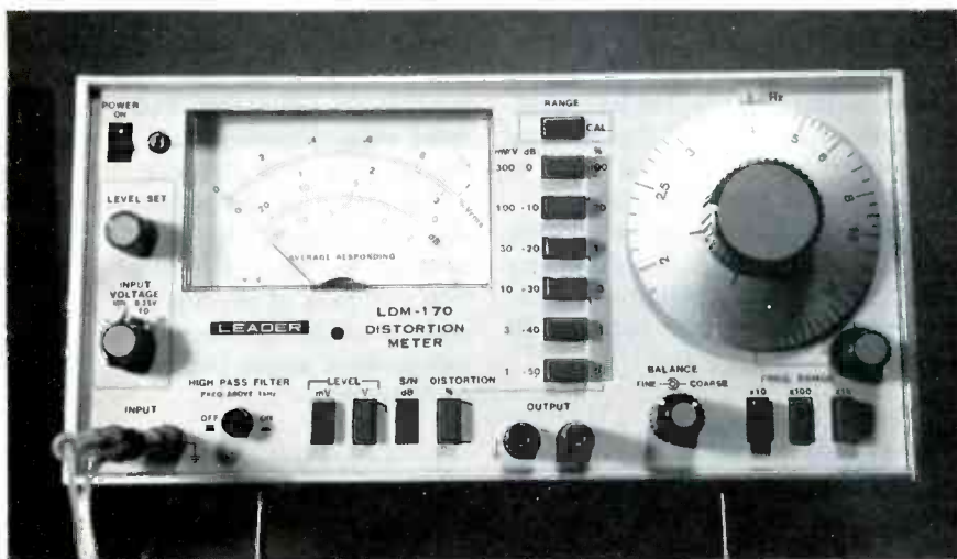
Fig. 3 Leader Model LDM-170 measures percentage of sine wave distortion, and also measures millivolts/volts RMS AC, or signal-to-noise ratio.
